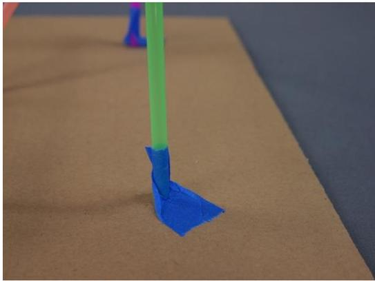
Uprights: Tape the straw to the cardboard so half the tape is pressed flat against the cardboard and the other half is pinched around the straw.
